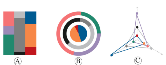
Fig. 6. Three design alternatives for the glyph where the proportions of presentation techniques are encoded by: (A) a treemap-based design; (B) a nested pie chart design; (C) a radar chart design.
